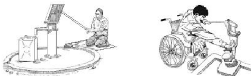
Figure 13: Example of accessible hand pump with concrete platform (Source: WEDC 2005)
