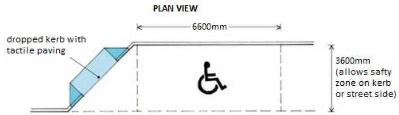
Figure 7: Floor plan of on-street access parking with kerb ramp (Source: Centre for Accessible Environments and RIBA 2004)
