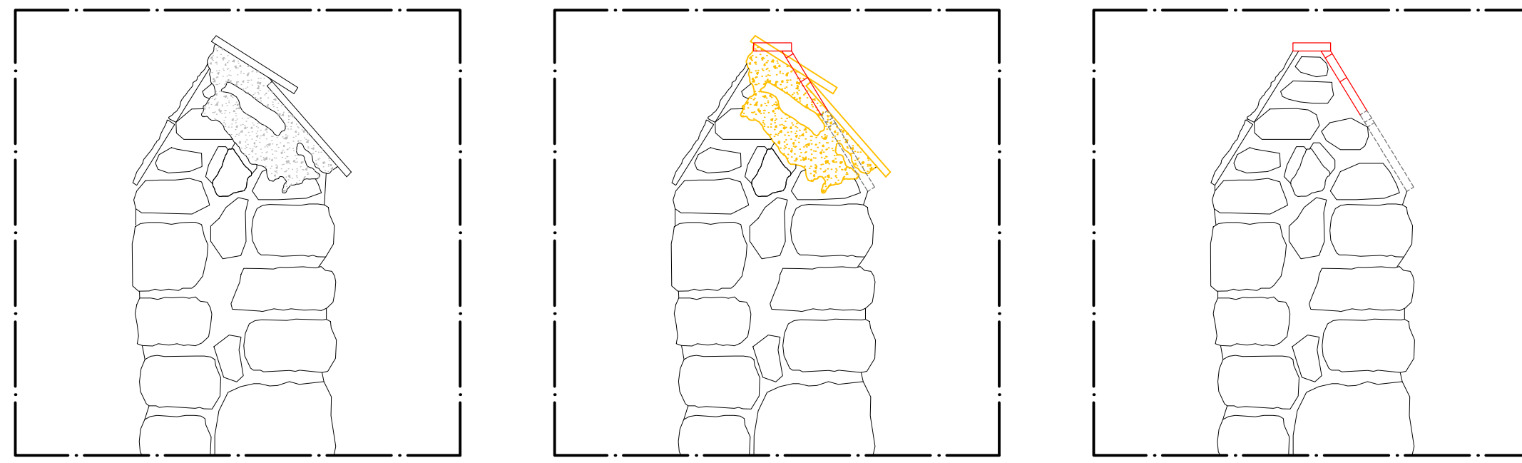
DETAIL 03. OPERATING SEQUENCES FOR THE INTERVENTION OF THE BATTLEMENTS - 1:20
